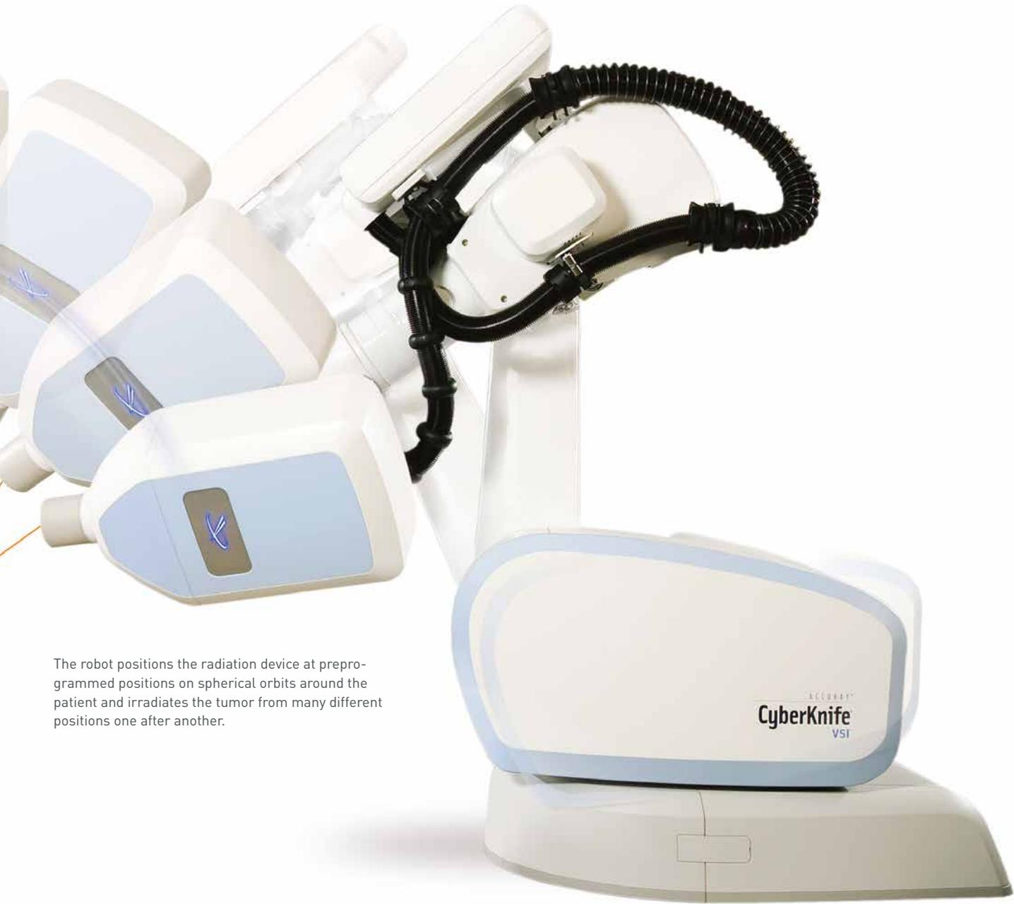
The robot positions the radiation device at pre-programmed positions on spherical orbits around the patient and irradiates the tumor from many different positions one after another.
